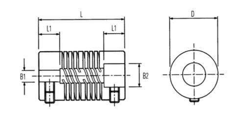
B1: Pre-drilled= 5.0B2: Pre-drilled= 8.00D= 25.4L= 38.1L1= 11.0Max angular displacement= 0.38Max B1 & B2= 12.70Max parallel displacement= 7
